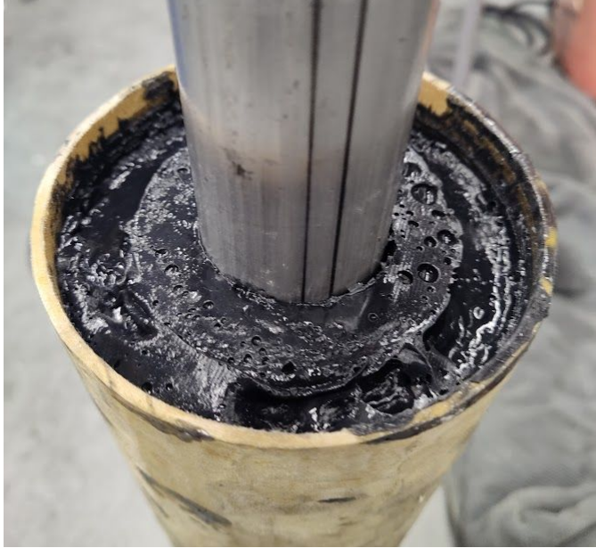
Fuel grain sank during curing
