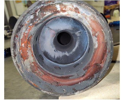
Nozzle Shear at RR plane
