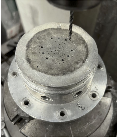
Adding 6 x \frac{1}{8} " holes to injectors
