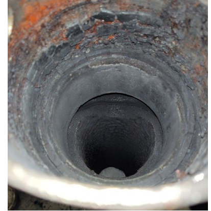
Severe ablation at grain - Post CC seal
