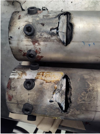
Burnthrough on both engines at post CC - nozzle interface
